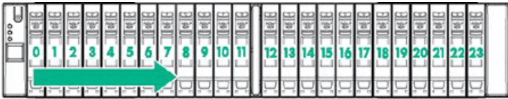
Figure 1: 3PAR StoreServ 8000 Storage 2.5-inch Drive Enclosure drive placement order
