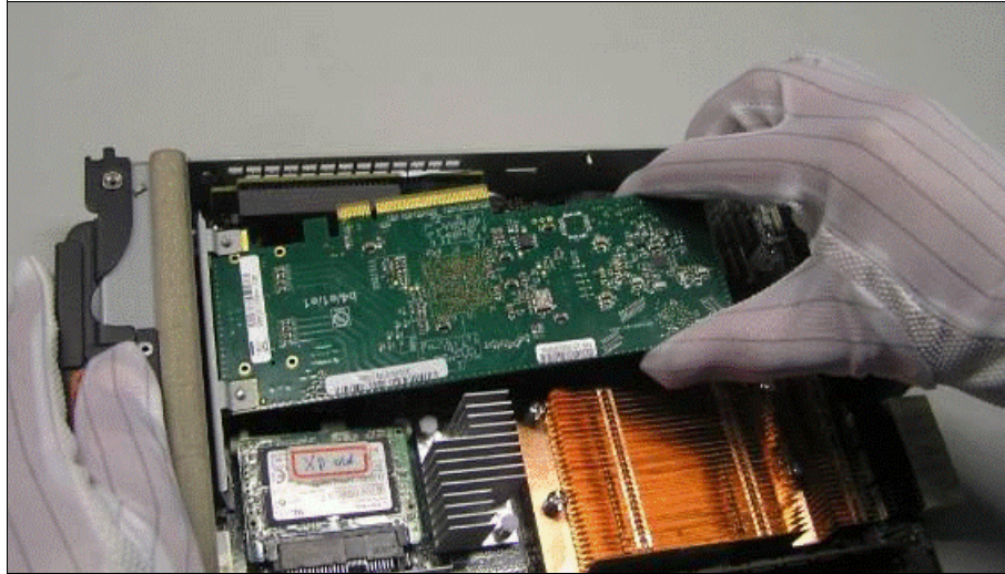
Figure 11-10 Host Interface card replacement
