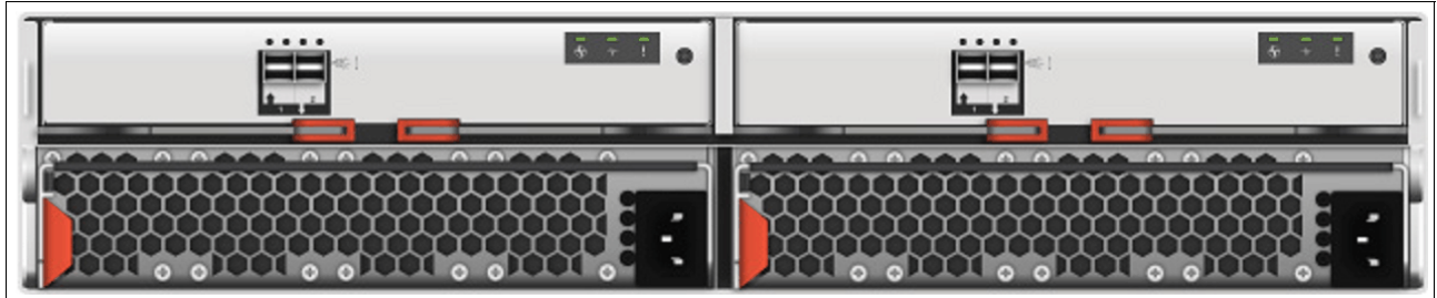
Figure 1-7 Expansion enclosure of the IBM Storwize V3700
