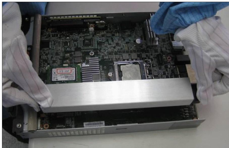
Figure 11-13 BBU replacement: Step 2
