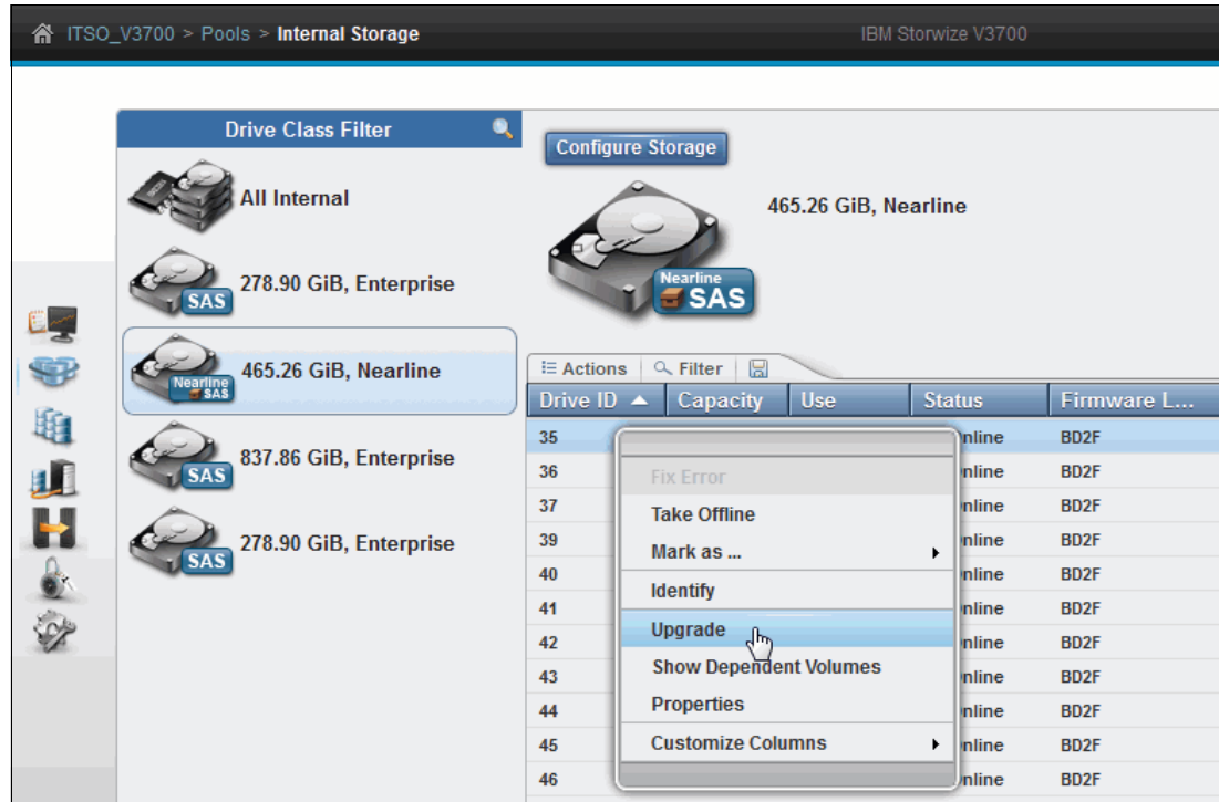
Figure 11-50 Upgrade an individual drive
