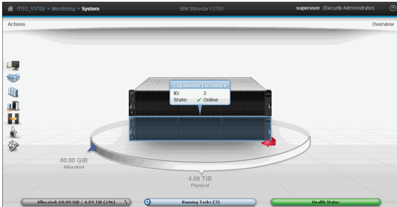
Figure 2-43 Expansion Enclosure included
