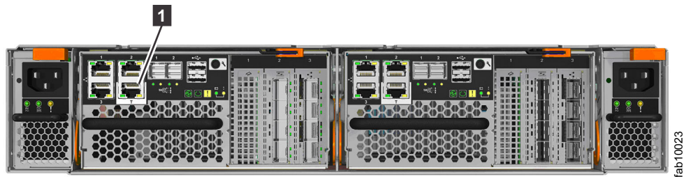
Figure 29. Storwize V7000 technician port
