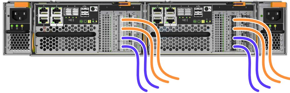
Figure 26. Example configuration with four Fibre Channel cables per canister
