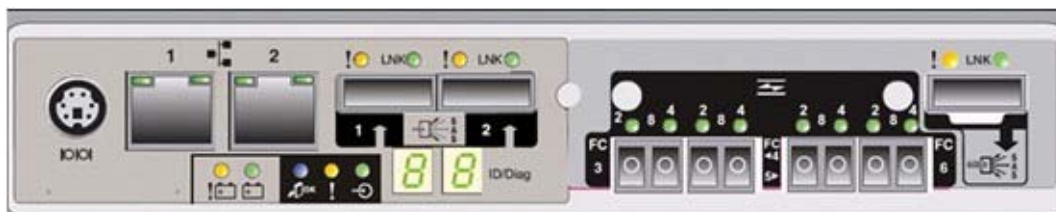
Figure 7. DS3500 controller rear view with FC daughter card
