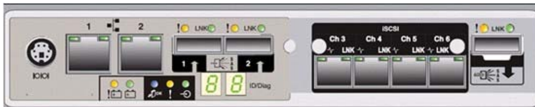
Figure 6. DS3500 controller rear view with iSCSI daughter card
