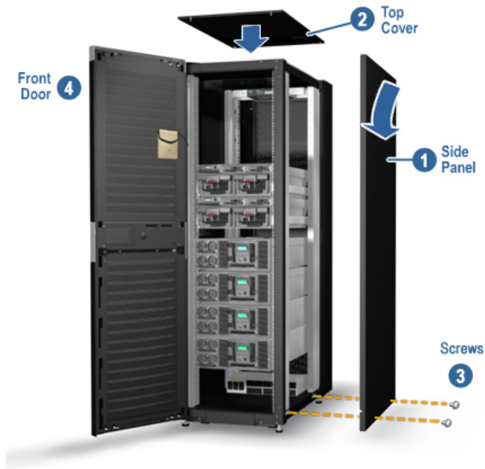
Figure 3–10 Replacing the Side Panel
