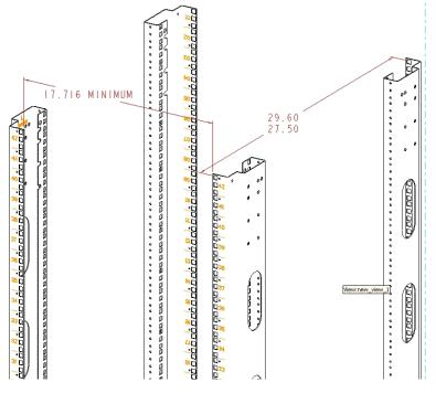
Figure 35 Mounting space dimensions
