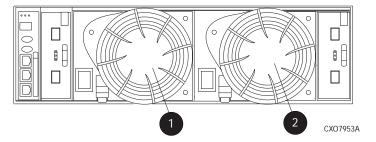
Figure 29 Blower element numbering
