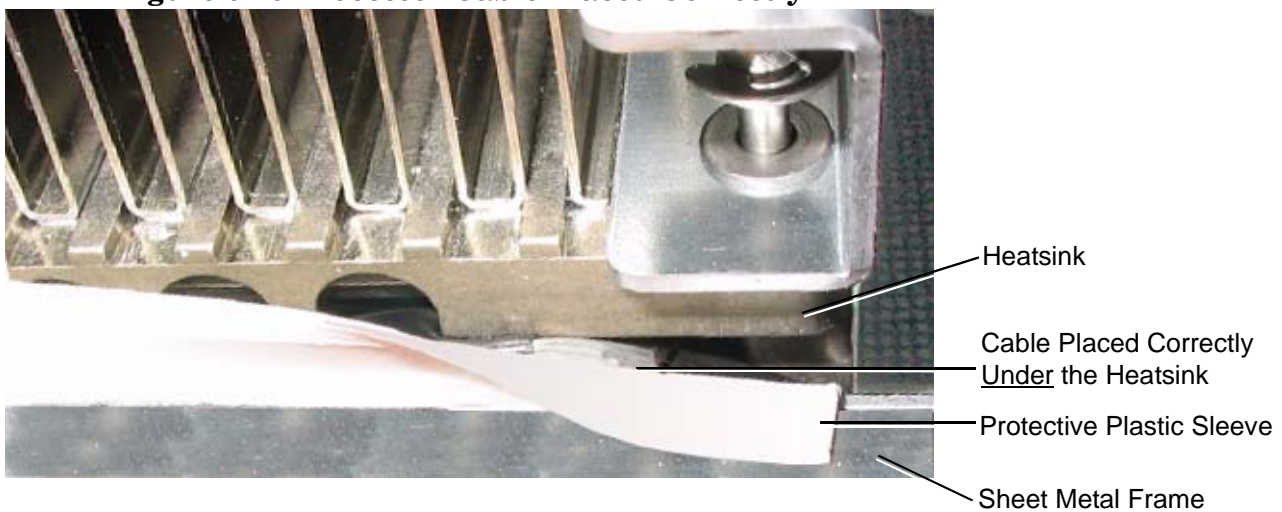
Figure 6-16 Processor Cable Placed Correctly
