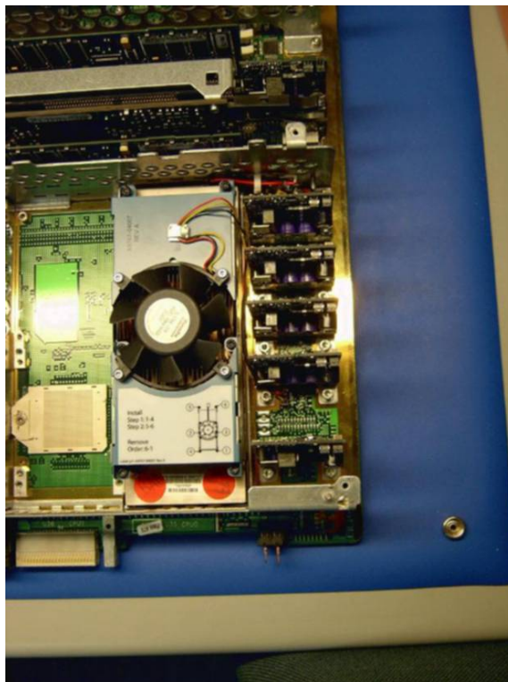
Figure 6-34 Sequencer Fan Assembly Installed
