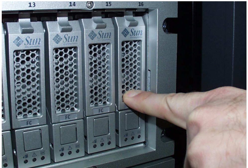
FIGURE A-2 Successfully Inserted Disk Drive
