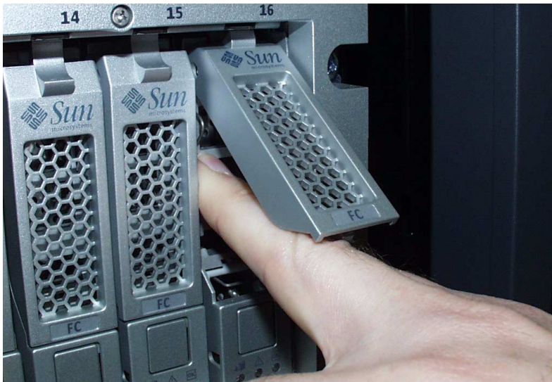
FIGURE A-3 Incorrect Method of Inserting a Hard Drive
