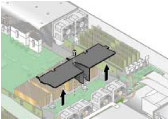
FIGURE 3-10 Removing the Center Air Baffle
