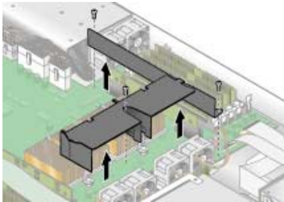
FIGURE 3-19 Removing the Center and Side Air Baffles
