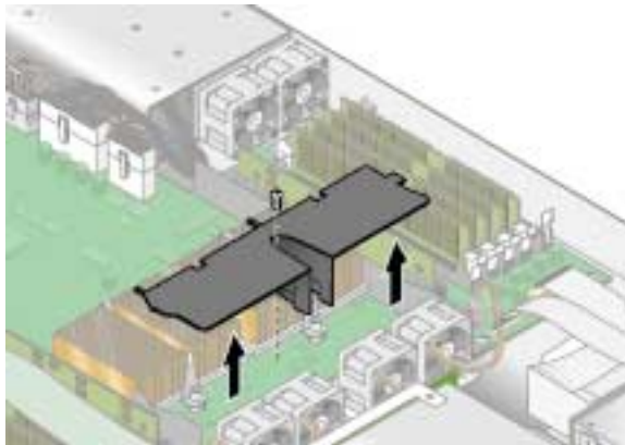
FIGURE 3-22 Removing the Center Air Baffle
