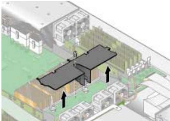
FIGURE 3-30 Removing the Center Air Baffle
